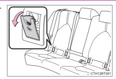
4 Check the positions of the exclusive fixing bars, and install the child restraint system to the seat.
