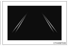
Indicates that the system is recognizing white (yellow) lines or a course\*. When the vehicle departs from its lane, the white line displayed on the side the vehicle departs from flashes yellow.
