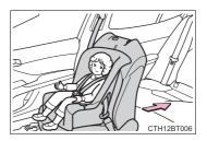
• Vehicles with front passenger occupant classification system: A forward-facing child restraint system may be installed on the front passenger seat only when it is unavoidable. When installing a forward-facing child restraint system on the front passenger seat, raise the seatback as much as possible, move the seat to the rearmost position, and raise the seat to the highest position, even if the "AIRBAG OFF" indicator light is illuminated.
