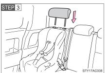
Reinstall the head restraint.
